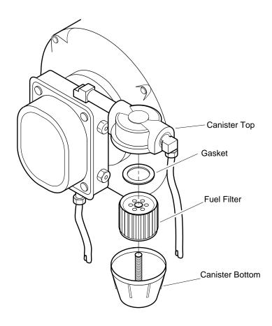
Figure 16 - Fuel Pump Filter and Canister
